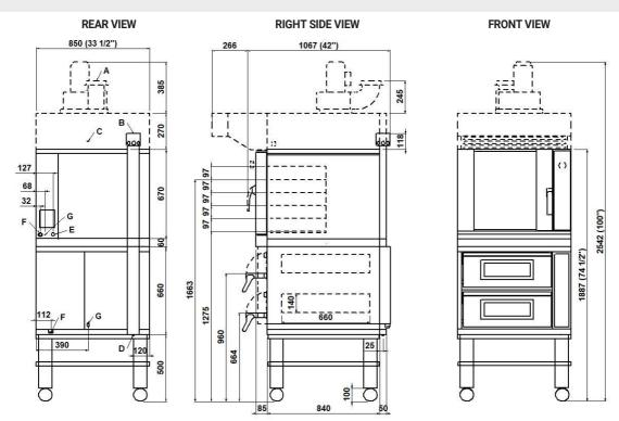
NOTE: The dimensions indicated in the views are in millimeters.
