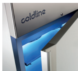
Door locks and stops Reversible door with lock and self-closes below 105° and stays open above 105°.
